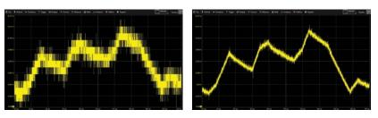
Comparison of 20-to-1 vertical zoom of a measured current signal from a pulse-width modulated inverter/drive output.
